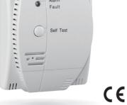
I-9602LW Addressable Gas Detector is used to detect leakage of home use combustible gas (LPG, Natural Gas) in such areas as houses, hotels and apartments. When leakage is detected, the detector will generate high buzzer alert sound, and provide a dry contact to turn exhaust fan, a 12VDC source to switch off the gas valve.
