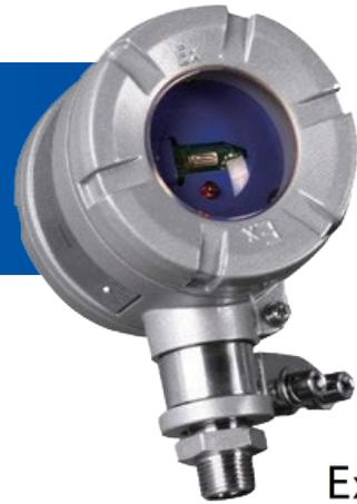
DI-9104Exd detects fire by picking up the ultraviolet light from flaming material. It's designed for areas where an open fire is liable to occur due to a large amount of radiation and no smoldering stage. This detector can be applicable to zone 1 and 2 of explosive areas.
