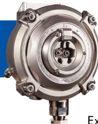
D-9107RExd uses two pyroelectric infrared sensors to detect the change of light signal of flame and background light signal at two bands of infrared spectrum through individual processing channels. The detector is applicable to explosive Zone 1 and 2, and flammable dust atmosphere.
